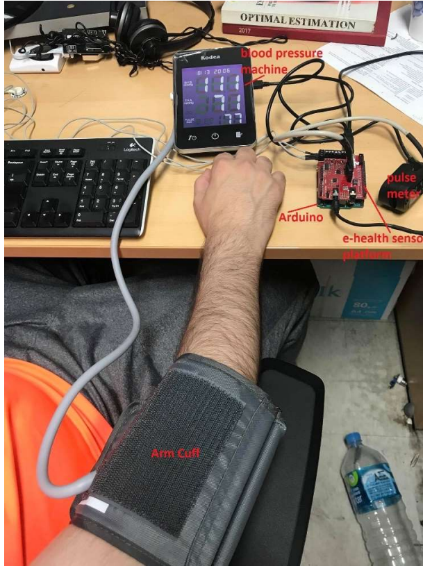
Fig. 4. Arduino setup with blood pressure sensor device.
